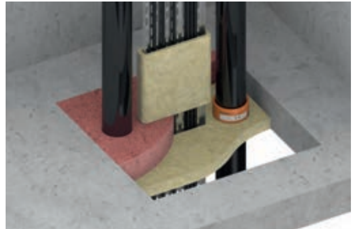
QF2 Fire Protection Compound used in conjunction with MW Mineral Wool Slab and QWW Intuwrap
